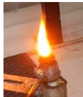
Figure 4 (left). Incomplete partial discharge when supplied with rectified current. U = 600V, R b >> 100 ohm
